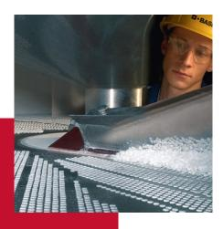
BASF is the first company worldwide to offer TPP as pellets (photo). Compared to the traditional flakes, this product reduces dust formation, prevents caking, improves handling and processing and is an improvement on safety.
